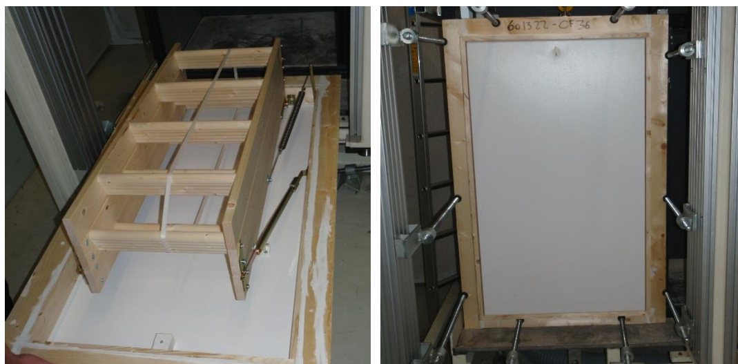
Loft ladder before and during testing
